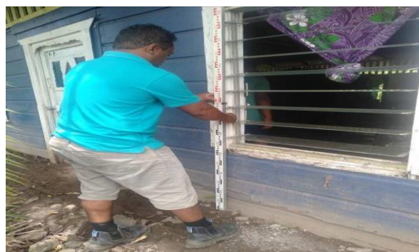
Flood Mark Survey after 18 th Dec 2020 Flooding Event
